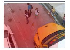
A predictive warning system combines radar, analytics, and integrated video in order to provide advanced audio/visual warning to both drivers and students that a motorist will likely not come to a complete stop during loading or unloading.
