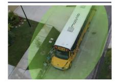
Exterior vision systems with intelligent analytics provide school bus drivers with audible and visual notification and verification of any students that may be directly around the bus prior to departure.
